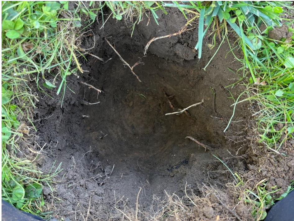
Image 10: Open Test Pit showing Subsurface Stratigraphy.
