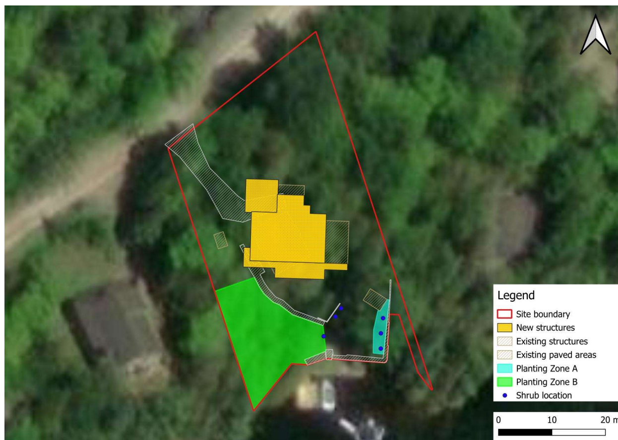
Figure 1: Site plan and planting locations on-site. 'Planting Zone A' (blue) represents areas suitable for planting shrubs and moisture/light tolerant wildflower species. 'Planting Zone B' (green) represents areas suitable for woodland flower and herb planting.
