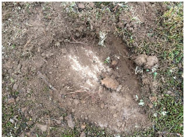
Image 24: Example of test pit with near surface bedrock in Southern Zone 3.
