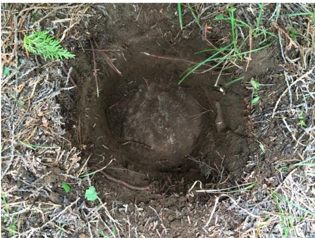
Image 23: Example of test pit in Southern Zone 3 with bedrock termination.
