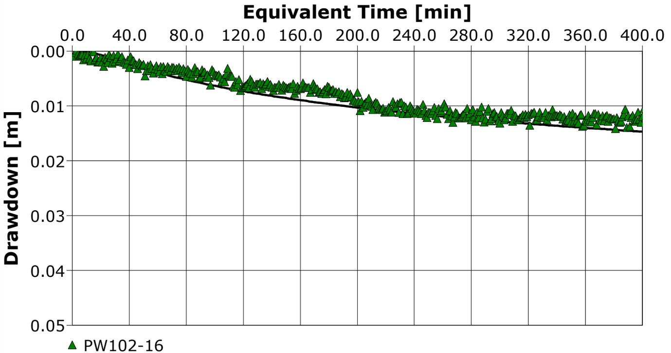
Calculation using Double Porosity
