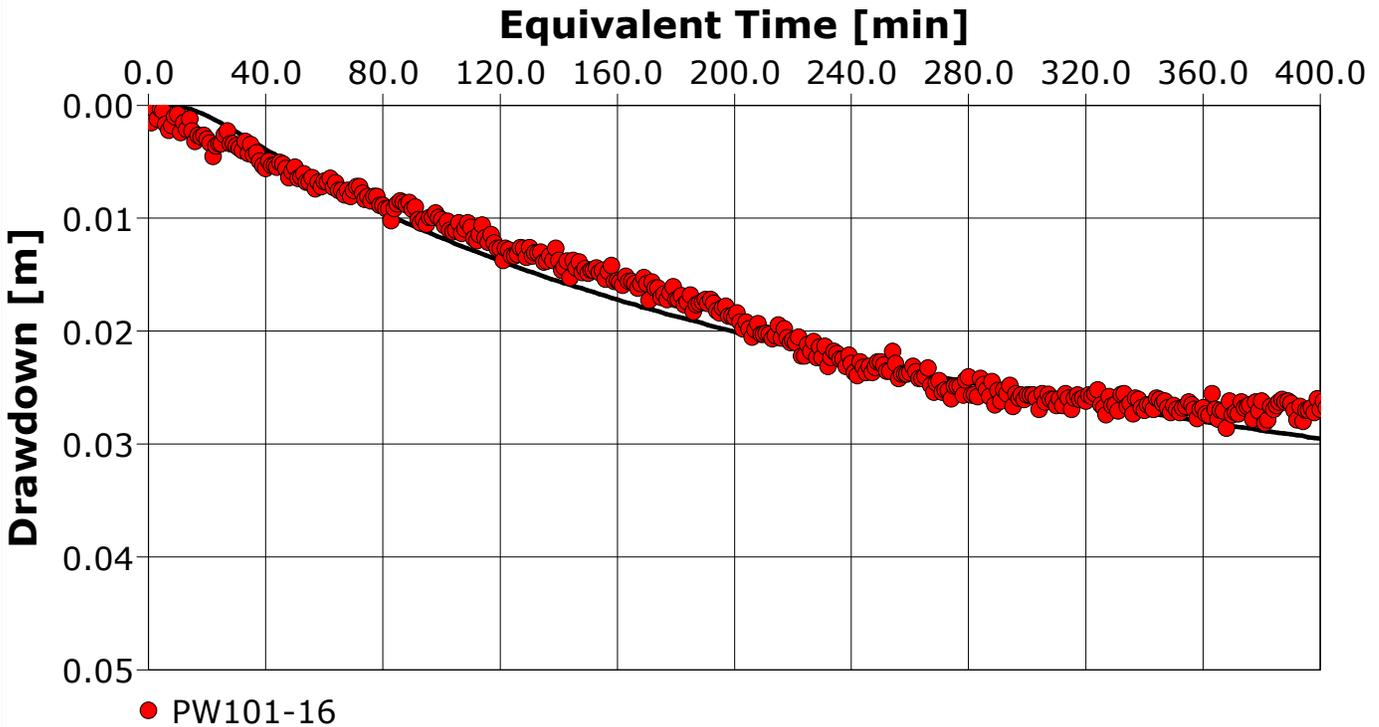
Calculation using Double Porosity
