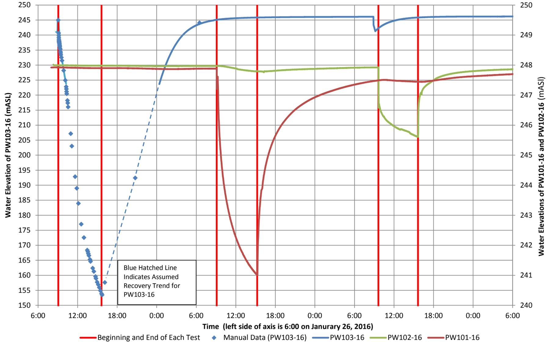
**Figure 3. Water Elevations of Pumping Wells**
