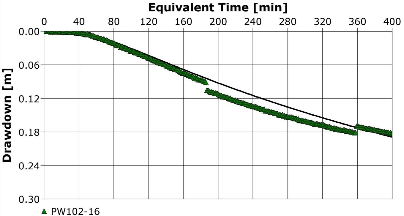
Calculation using Double Porosity
